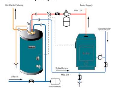
Alliance SL water heaters have a higher recovery rate than typical direct fired or electrically operated water heaters because they utilize the large output from the boiler as the heat source.
