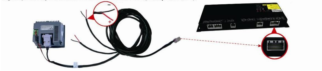
Pic 6-8 Screen Connects to EK-YT-M2124 Module with Communication Line
