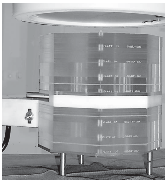
Figure 1. The NEMA Cardiology phantom
