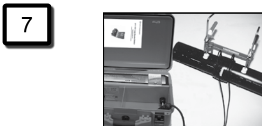
7 Connect welder to clamped assembly and follow welding unit instructions. Ensure appropriate welding cables are used.
