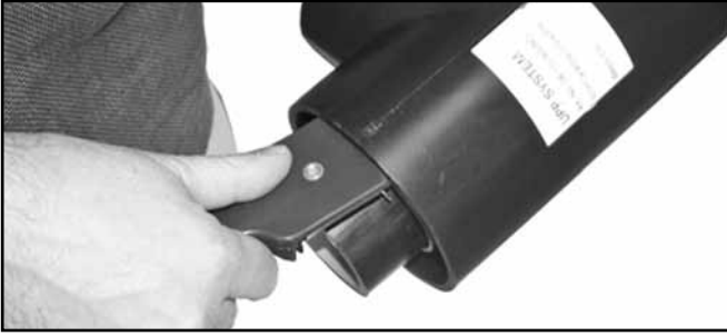
Scrape Primary and Secondary
