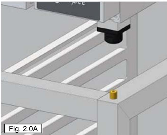
Install the appliance in a position that allows access to the right side for installation, maintenance and technical assistance.
