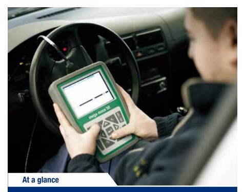
Using the mega macs 50 a technician can solve problems with a modest amount of time and effort using the key pad designed to keep the number of button depressions to a minimum. The mobile tester helps with systematic troubleshooting and completes your diagnostics by depicting all important parameters in both diagrams and numbers. Mega macs even converts the data transmitted in the vehicle, via CAN-bus, into information for evaluation.
