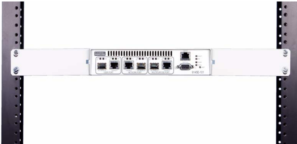
Figure 3-4. Mount 9145E on Rack
