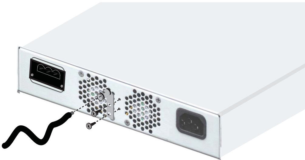
Figure 3-12. Install Grounding Lug
