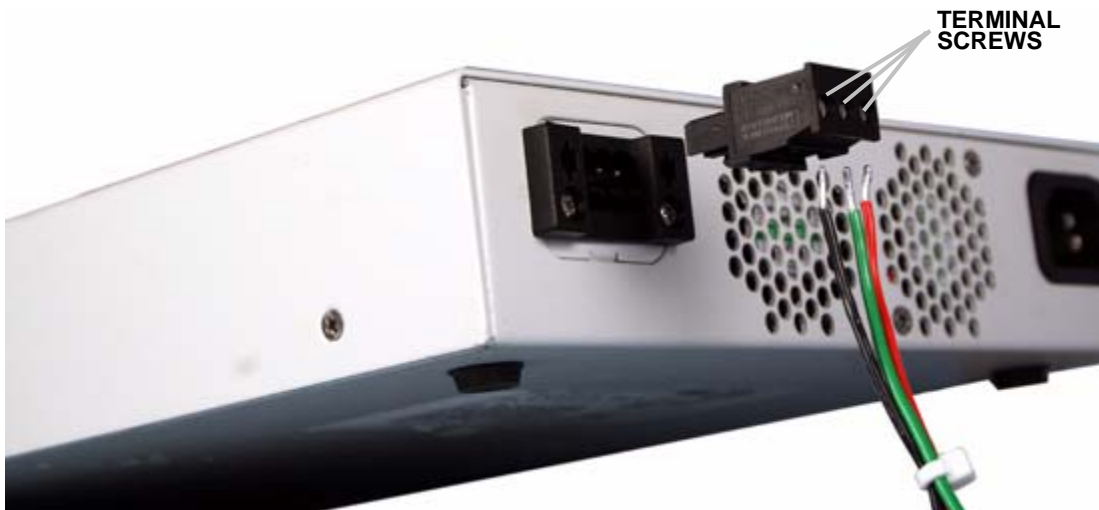
Figure 3-11. Connect D.C. Power
