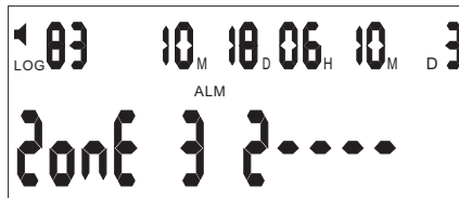
Figure 10: The LCD display when the wired detector is alarming
