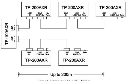
Figure 4: Connecting Multiple Devices
