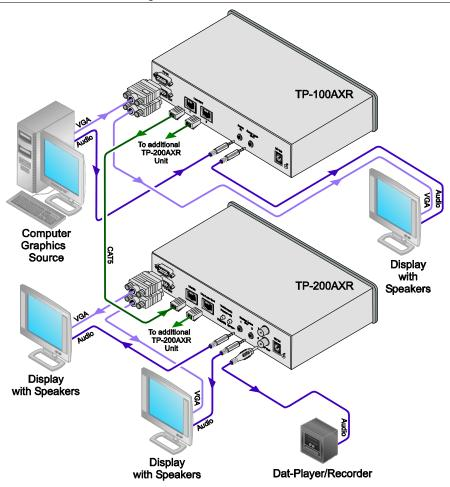
Figure 3: Connecting the PC/Audio Line Transmitter/Receiver System
