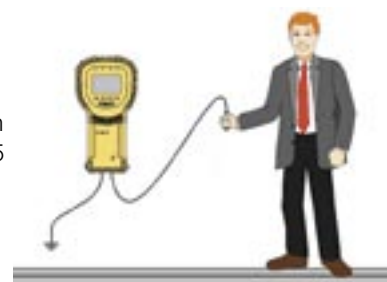
R_E system resistance test set-up.
