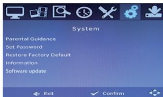
To access the Menu, press MENU and select [System]. The menu provides options to adjust the system settings. Press the UP/DOWN key to select an option and press RIGHT/LEFT to adjust the setting. Press EXIT to exit the Menu.
