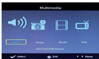
From the multimedia menu you can access information stored in an external device connected via USB. When a USB device is attached you can select from the Music, Photo, Movie or PVR options in this menu using the RIGHT/LEFT keys and OK to select. If a USB device is not connected, the warning message "No USB device is Found" will appear.
