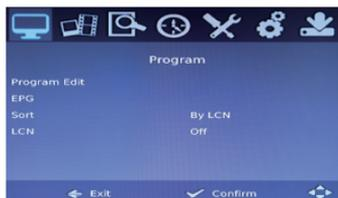
To access the Menu, press the MENU button and select [Program]. The Menu provides options to adjust the Program Settings. Select an option and press OK or RIGHT to adjust that setting. Press the EXIT button to exit the Menu.
