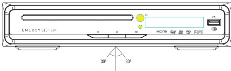
The remote control will not operate if its path is blocked.
