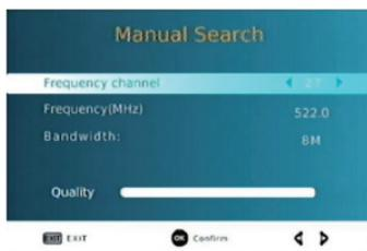
Install new channels manually. This option adds new channels without changing the current channels list.
