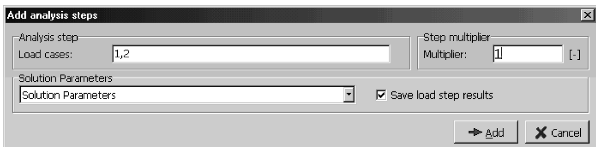
Figure 52: Each step will be composed of load cases 1 and 2. The multiplier 3 will be used to multiply the applied actions and the newly created solution parameters will be used during the load steps.
