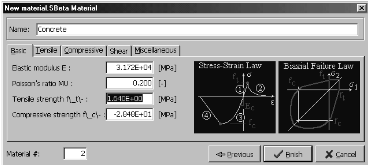
Figure 12: The dialog window for the definition of basic properties for SBETA material. The parameters were generated based on the concrete cube strength. The tensile strength should be edited to 1.64 MPa for the Leonhard's beam.
