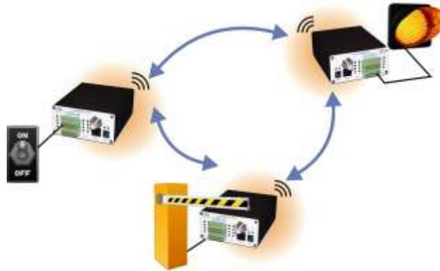
Example application: Wireless ON/OFF switch control
