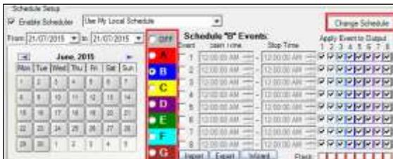
3. Place a check mark in the event number that is to be used. This will enable the start/stop time to be added for the event. Select the desired start/stop time for the event.
