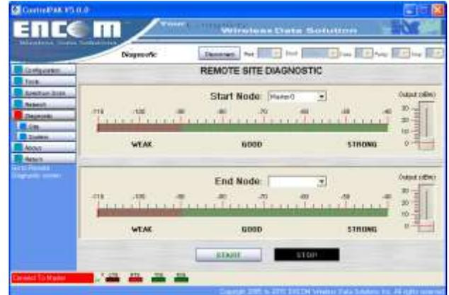
The red and green bars indicate the power of the signal currently being received from the other radio. The two sliders on the right side of each panel control the output power on the Radios. This slider should be lowered if the signal strength is too strong and raised if it is too low.
