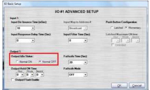
(Please be aware, after changing the output from "Normal OFF" to "Normal ON", the corresponding output status LEDs will also be inverted)
