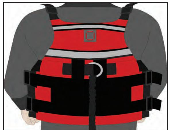
1. Open the fix lock buckle and un-thread the webbing belt through x4 webbing loops on the PFD (Personal Flotation Device).
