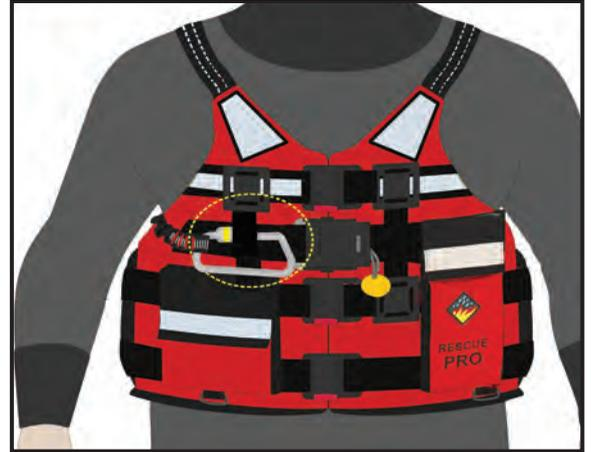
When the cowtail is not in use ensure you clip the karabiner into the quick release mechanism located on the front of the PFD as illustrated. (see illustration in fig 7)
