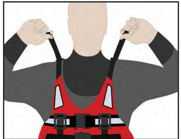
Finally take the two shoulder straps and pull forward simultaneously to ensure the correct adjustment. The personal flotation device should fit snug around the body.
