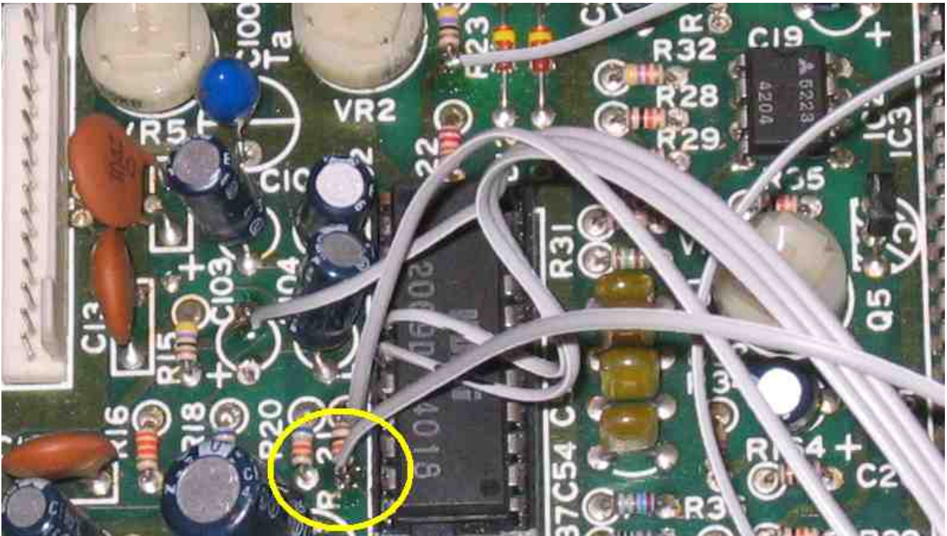
Illustration 16: The Connection from Pin 21 on the AtomaHawk to Resistor R21 (lower side)
