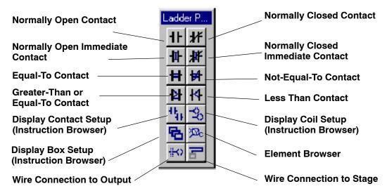
Use the **Ladder Palette** to enter the first instruction of the program. First move the cursor to the desired location of the first element. A normally open contact needs to be placed in the selected position to load the preset on the first scan. To do this, click on the button that shows the normally open symbol. This will open a small input window for setting up the contact.
