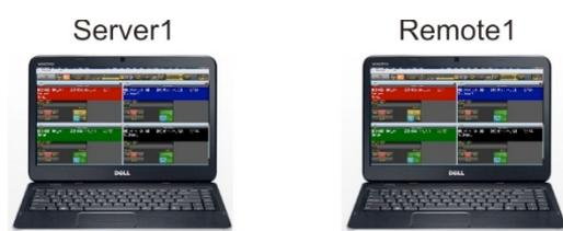
The Audio Console Server - a part of the SCENEFLOW Pro system - is installed on Server1. It manages and replays the audio files and it has an audio interface installed. The Remote1 computer runs the Remote GUI of SCENEFLOW Pro. This configuration is useful when the mixing console and the playback system cannot be in one location. There are more details [here](#).
