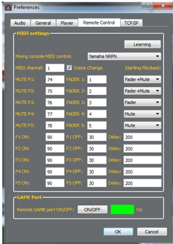
Connect the console with the computer either using the MIDI port on the audio interface or using a special MIDI/USB interface. Before you start to set up the MIDI functions, we suggest to check the mixing console settings:
