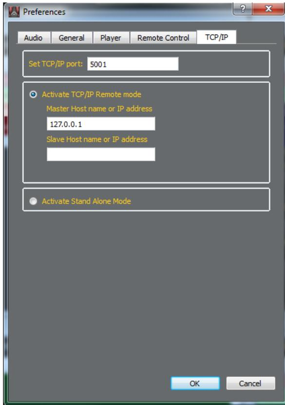
Use the Standalone mode if you are using the system on one computer without Remote control. Select the Standalone mode switch and click OK. After SCENEFLOW is launched, the engine playing the audiofiles is automatically launched locally and no Remote control stations can be used for the user interface.
