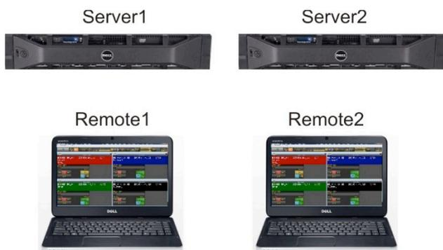
The Audio Console Server - a part of the SCENEFLOW Pro system - is installed on Server1 and Server2. It manages and replays the audio files. Both Servers have audio interfaces installed. Remote1 and 2 computers run the Remote GUI components of SCENEFLOW Pro. Remote GUI controls both Servers synchronously, so any failure of one server does not harm the production and the other Server may continue playback. There are
