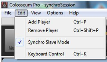
In this menu, only disconnection is available. To start the whole system in the Master-Slave mode, you need to close the project and open it with the parameter Sync Slave Mode in the Open Project menu of the main menu bar.
