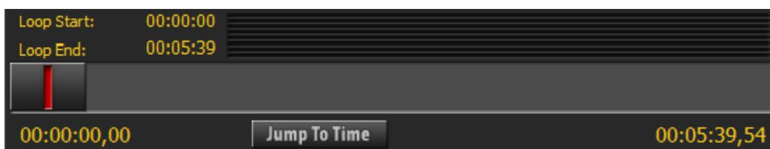
The track slider and the “Jump To Time” button allow to move the playhead to any position in the track or to a position inside the loop if the loop is active.
