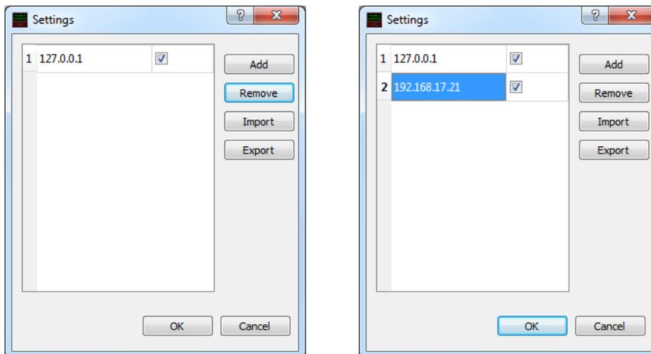
5. Click „**Add**“ and fill the IP address of the Audio Console server (visible in the window with the **No Access** message) and press „**OK**“.
