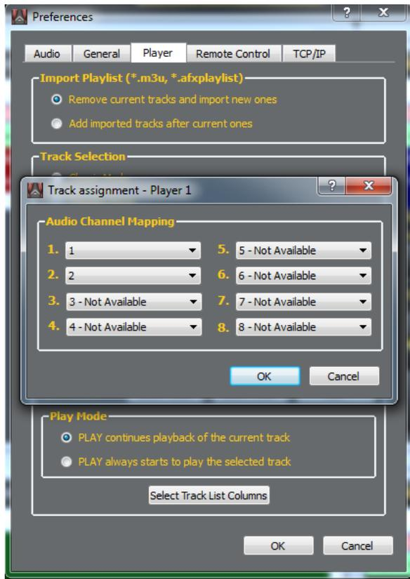
Click the “Edit” button. The Audio Channel Mapping dialog appears, assign the player outputs to the available channels of your audio interface. Assign “Not connected” to the unused channels
