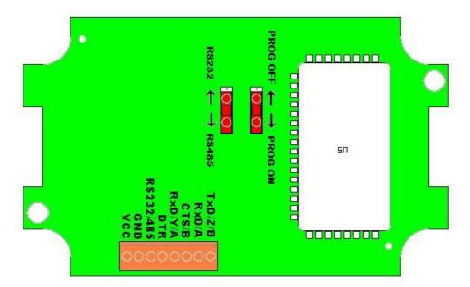
> TxD, RxD: Serial link signals in RS232 format. TxD is for the data going out of the Terminal
