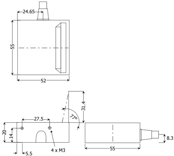
Note: To prevent infiltration of dust or other contaminants into the scanner through the mounting holes provided in the unit's case, short screws (M3-6) may be placed in each hole location. The shafts must not penetrate into the case further than 0.25 inches (6mm).
