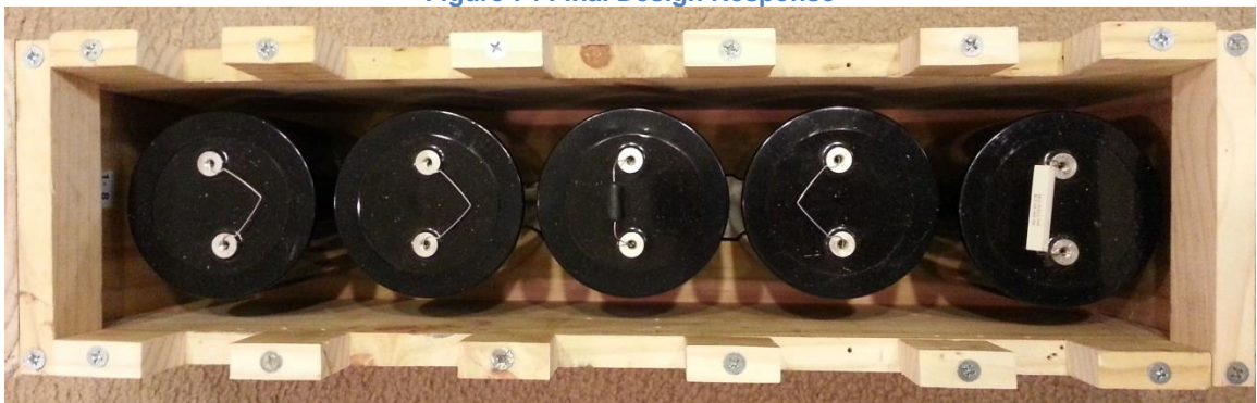
Figure 75 Capacitor Bank. 5 capacitors Top down view.
