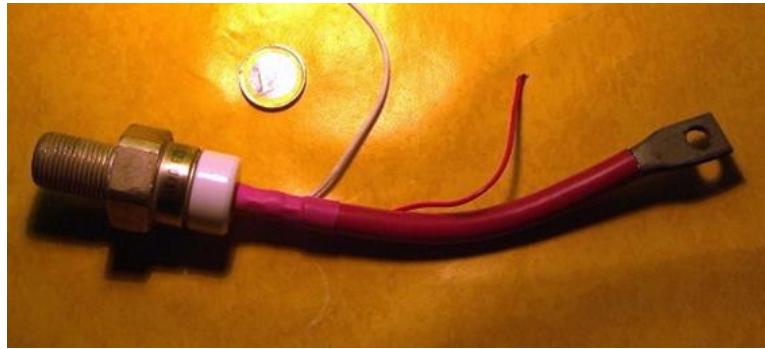
Figure 10 Silicon Controlled Rectifier, Reprinted with permission from Antonio Pedreira
