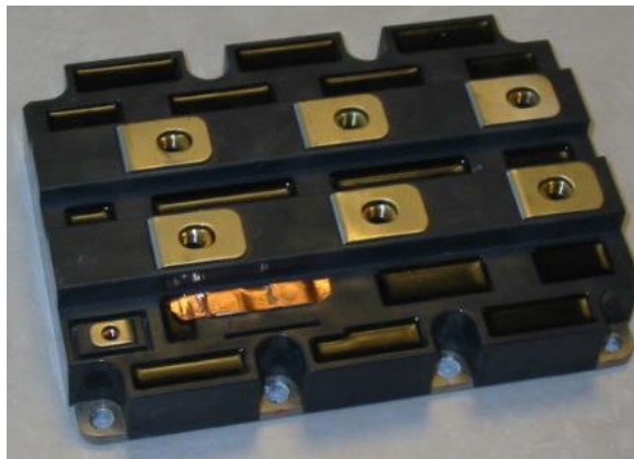
Figure 13 Insulated Gate Bipolar Transistor. (Reprinted under permission of the GNU Free Documentation License and Creative Commons Attribution-Share Alike 3.0 Unported license)
