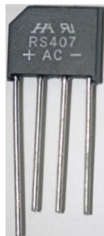
Figure 32 Bridge Rectifier. Reprinted with permission from user "Metaresephotos" under the Creative Commons Attribution 3.0 Unported license
