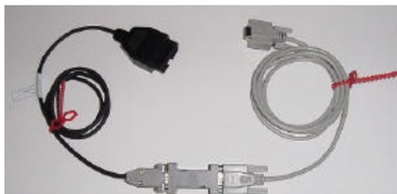
Vehicle Communication Cable for Visteon ECU/ECM
