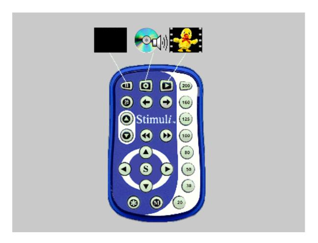
The Video Play button controls playing and stopping of video clips. When a video clip is playing the Up (a) and Down (c) Circle buttons and the Direct Access buttons control selection of additional clips.
