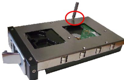
**step 3.** Press tray handle on Sliding the tray with hard drive into the enclosure
