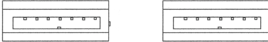
Figure 3: Using SeriTek/e6G with a drive enclosure that has L-shaped eSATA connectors; both cable connectors will be identical.
