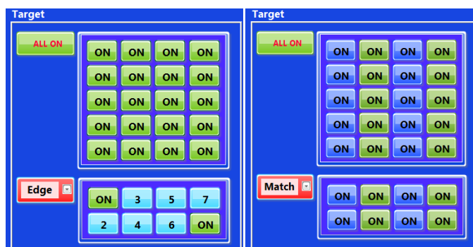
Figure 22. Gate 1 and 8 are always ON (left side); only the two Gates belonging to the same column as the DUT are energized (right side).
