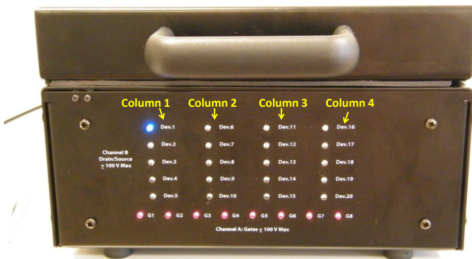
Figure 8. The Multiplexer Measurement Unit addresses Devices by assigning Device columns.
