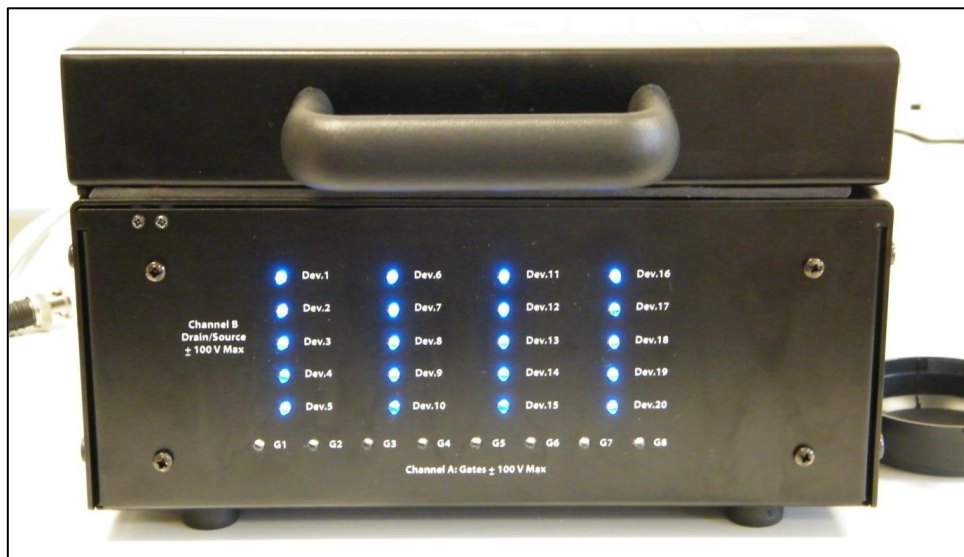
Figure 10. The Multiplexer Measurement Unit used for stress biased acquisition.
