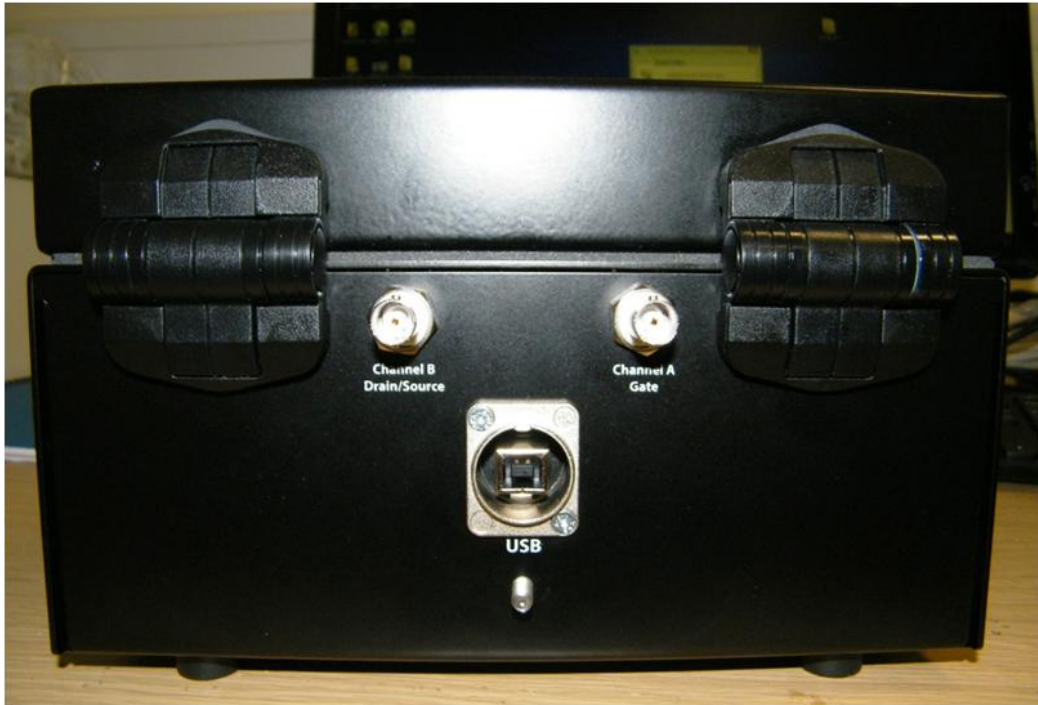
Figure 1. USB cable and coaxial cables (BNCs) connection: Channel A is the Gate; Channel B is the Drain.
