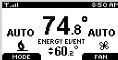
During periods of high electricity demand, a Blue LED will illuminate on your thermostat and your Setpoint name will be replaced with "Energy Event". This indicates that the Setpoint temperature has been adjusted to save energy and the new target temperature will be displayed below the words "Energy Event".
