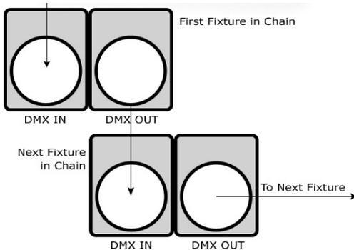
**A quick note:** Often, the setup for Master-Slave and Standalone operation requires that the first fixture in the chain be initialized for this purpose via either settings in the control panel or DIP-switches. Secondly, the fixtures that follow may also require a slave setting.
