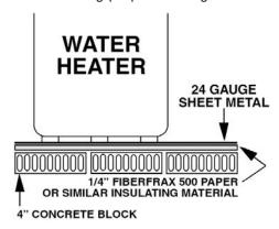
Minimum clearance to combustible construction is: SIDES 6"; BACK 6"; FRONT 24". The installation of this water heater must conform with local codes and ordinances. In the absence of local codes, the installation must comply with the National Fire Protection Association (NFPA 31) Code.
