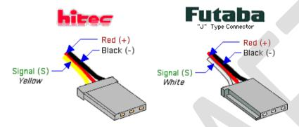
On the demo board, such servos are directly connectible to the pin headers. PWM1, 2, 4
