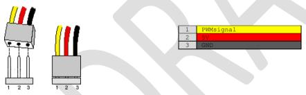
Always check with your specific servo brand if the wiring is respected.
