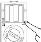
Open the battery cover of the Interior Unit and press and hold the **[Registration]** button for 5 seconds.
