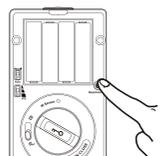
Open the battery cover of the Interior Unit and press the **[Registration]** button briefly.
