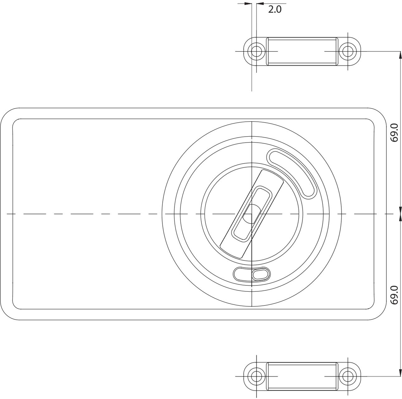
**Drilling Template Sheet for 70mm Backset**
