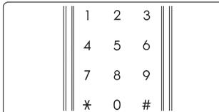
Press and hold the **[#]** button on the outdoor assembly for 3 seconds.
