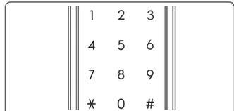
Enter the Master PIN Code or User PIN Code and press the **[\*]** button to set the security function.
