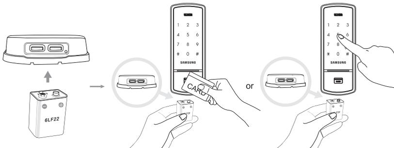
Continuing to use the lock without replacing the batteries when required will lead to lock malfunction. Touching a 9V DC battery to the external power contacts on the under-side of the Exterior Unit will allow for temporary access (continue touching the battery to the contacts until the lock is open).
