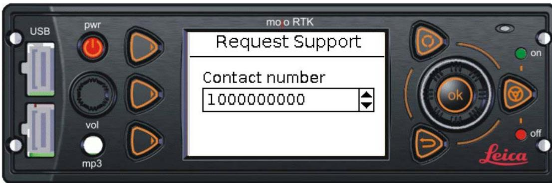
Use the main dial to scroll through the stored numbers and press the OK button to select a number. If you wish to add a new number use the main dial to select 'Add new number' and press the OK button. If a phone number has never been entered you will be taken directly to this screen.
