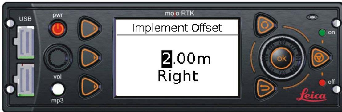
Press the OK button to use the new implement offset and return to the Guidance screen. Press the Escape key three times to return to the Navigation screen.
