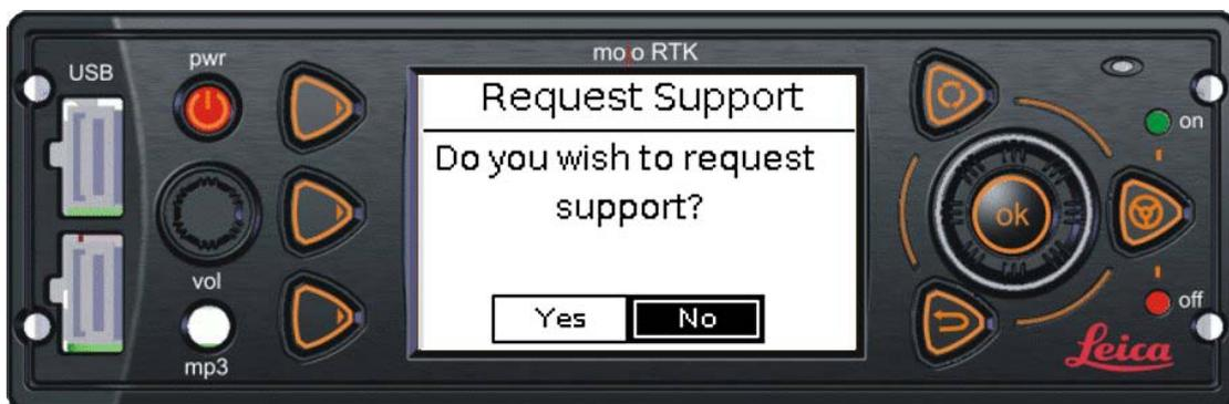
To request support rotate the main dial to select 'Yes' and press the OK button. If you have been instructed to connect to Virtual Wrench™ by a technician, you do not need to request support at this time so select 'No'.
