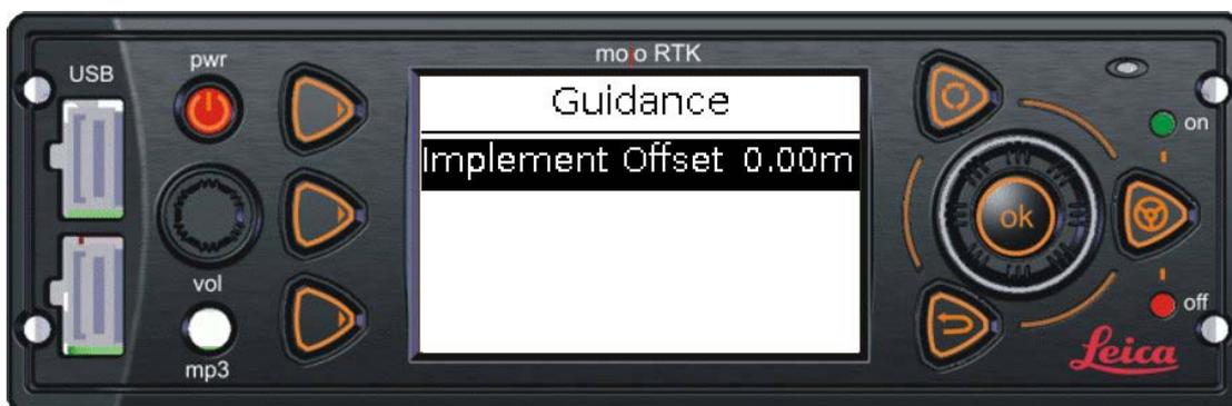
To change the implement offset, use the main dial to change the whole units first, rotating the dial clockwise to move the offset right or anti-clockwise to move the offset left. Once you have set the whole units to the desired value press the OK button, this will allow you to change the fractional units. Rotate the main dial to enter the fractional units. If you make a mistake you can go back by pressing the Escape key.
