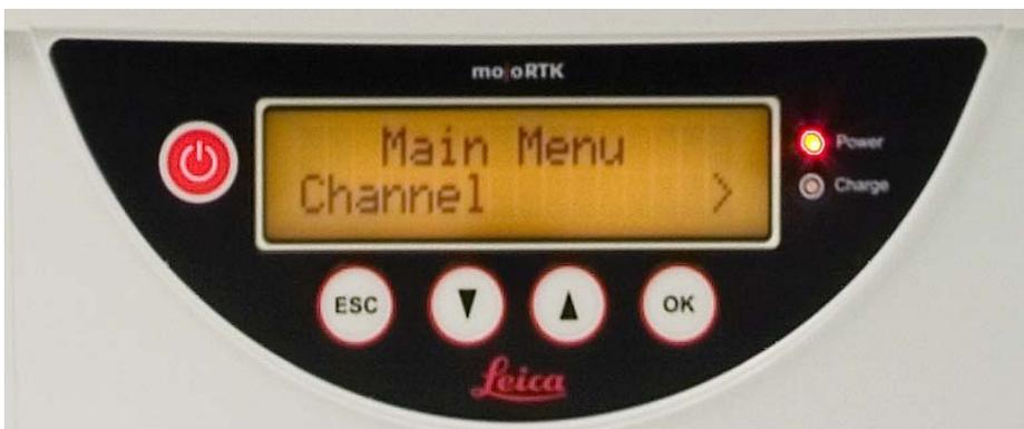
To enter the channel menu option press either of the up/down buttons or the OK button. The menu option 'Channel' will be displayed. If you are already in the menu system you need to scroll through the menu options using the up/down buttons until you reach the channel option.
