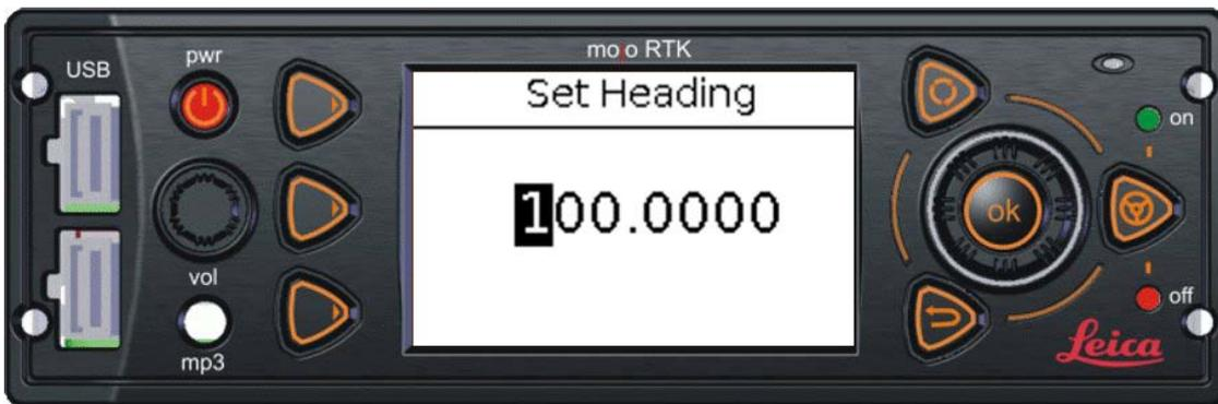
To enter the heading use the main dial to increase and decrease the currently selected digit. Press the Ok button to move to the next digit or the Esc button to move to the previous digit.
