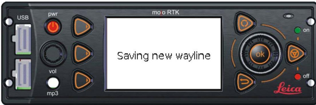
If you are setting an A-Heading wayline then after setting the A point you will need to enter the desired heading.
