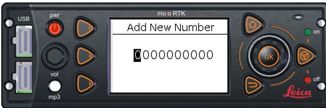
Use the main dial to change each digit. Press the OK button to move to the next digit or the Escape button to move back. Once you have entered the number press the OK button. The console will display a request for confirmation screen as shown below:
