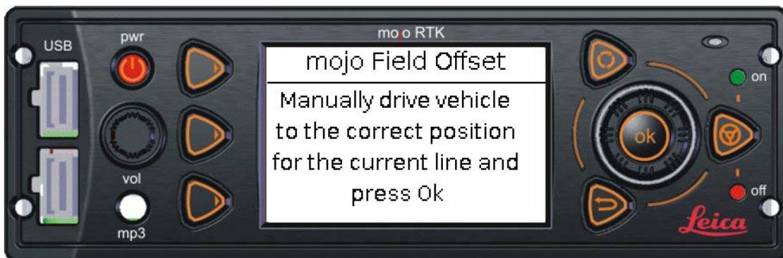
Once your vehicle is positioned correctly press the OK button.
