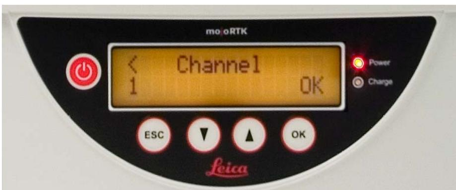
To enter a new channel, use the up or down button to select the desired channel number and press the OK button. The display will now read 'Channel changed' and after a short while normal operation will resume.
