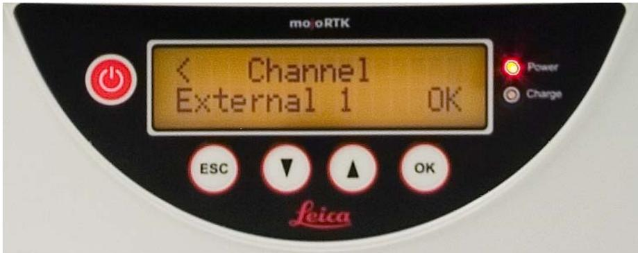
You will then be asked to choose the correct baud rate, which should be found in the user manual for your external radio. Use the up/down keys to select the appropriate baud rate and press OK.
