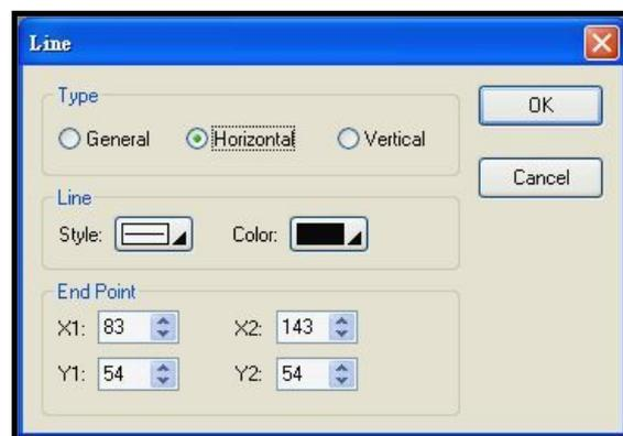
To change the length or the position of the horizontal lines, click the target line to see two checks at the ends of the line, move the cursor on the checks. After the cursor turns to a cross arrow, press the left button of the mouse and drag the line to any position you like on the working area.
