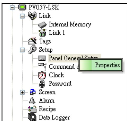
These settings are used when communicating with control devices. Actually, every setting should be set according to each application and device the HMI communicate to. And for the best performance, the settings should be set correctly. About the settings, please refer to local agents or our website for further information.
