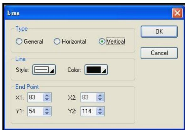
To change the length or the position of the Vertical lines, click the target line to see two checks at the ends of the line, move the cursor on the checks. After the cursor turns to a cross arrow, press the left button of the mouse and drag the line to any position you like on the working area.
