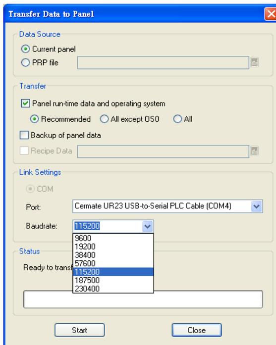
Figure 2-72 Panel menu\_ Transfer Data to Panel\_baudrate setting
