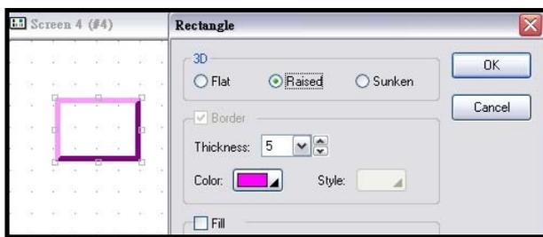
Click Raised to select Thickness and Color. The Border is not selectable. When a color is chosen, PanelMaster shows default coordinated dark color on the right and bottom of the rectangle.
