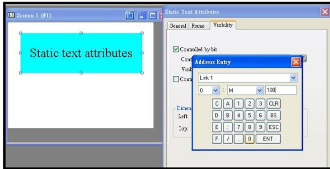
The text can be controlled by user level, too. There are 8 user levels. Click visibility to see the dialogue. Enter user level to complete the setting. In some applications, when the text contents should not be operated by users, set the text controlled by user level to protect texts. The higher user level can see the text by entering password.
