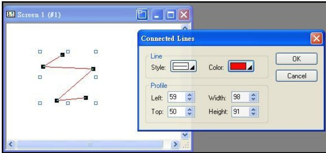
Click connected line button from the Tool bar, move the cursor to the the working area then click the left button of the mouse to draw the first point of a connected line. Move cursor to next point and so forth. After drawing a connected line, double click left of the mouse to design the line.
