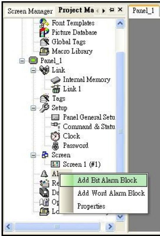
Set the Bit Alarm block before using Display the alarm message function. There are 16 blocks for setting. Please see below for your reference.
