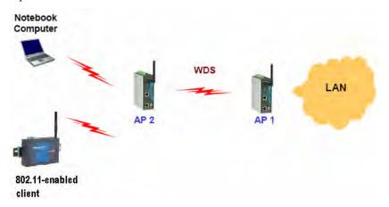
By using WDS, two or more LAN segments can be connected wirelessly. As illustrated in the above figure, a pair of wireless LAN-to-LAN bridges is used to connect two LAN segments. Since the AP is WDS-enabled, it can be used as a wireless bridge.
