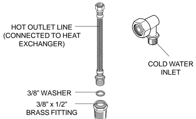
**Fig. 3 - Water connections**
