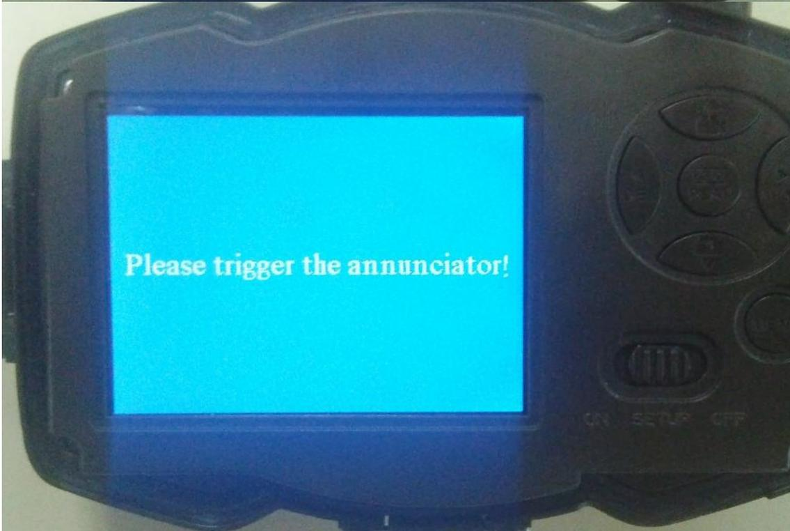
2. Power on or trigger the wireless sensor to study code.
