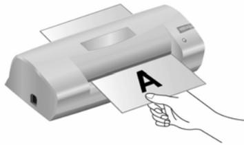
4. The scanner pulls the calibration sheet through the scanner, which completes this scanner calibration.
