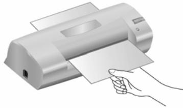
4. The scanner pulls the cleaning paper through the scanner, which completes this scanner cleaning.
