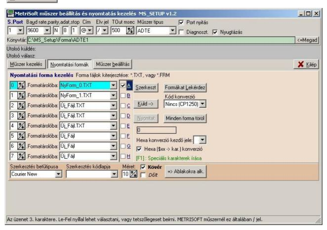
In MS-ADT1 instrument, 2 different printing forms can be stored. These forms can be placed in the 0. and 1. form containers. A printing form can be assigned to a container on the following part of the screen:
