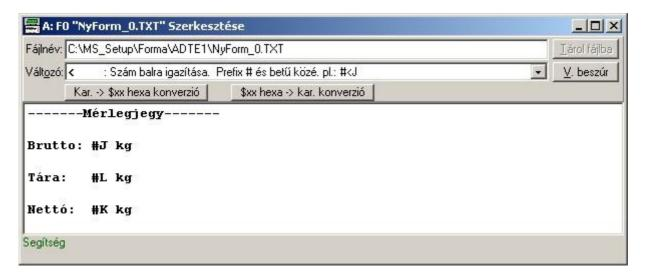
The window above has an edit box that is used to specify the appearance of the printig form. By giving any constant text content, it is possible to insert variable fields too, which have changing values during operation of the program (Examples: serial number, mass values, date). The variables are marked with a "#" sign and can be selected from this checkbox here below:
