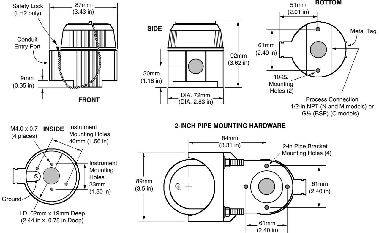
Figure 6. D-BOX Housing Dimensions (For use with the TDZ<sup>2</sup>)
