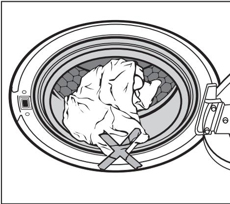
To prevent damage to the door seal and clothing, make sure that there are no clothes caught between the drum door and the seal.
