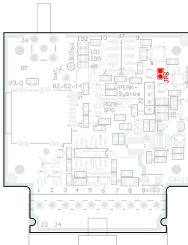
Solder field JP6 on the circuit board
