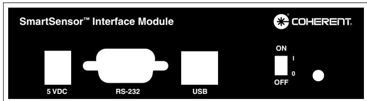
**5 VDC Power Input** – Connect the provided 5V Power supply. The power supply is designed for the following AC input requirements: 100-240V, ~0.2A, 50-60 Hz. The 5V input also provides battery charging capability for the SmartSensor Interface Module. When the 5V supply is connected to the Interface Module, the battery will be charging regardless of the power switch position. The USB connection does not provide battery charging capability.
