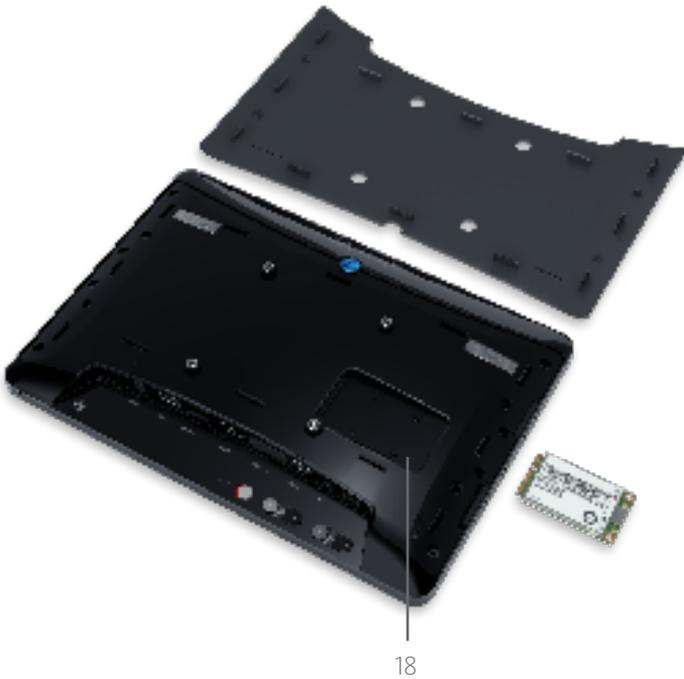
iDISPLAY Tablet 21.5" with back panel removed
