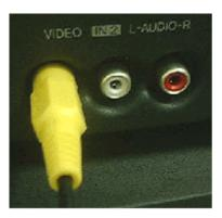
D1. Connect either the yellowtipped RCA composite video OR the solid black S-video cable (recommended) into the video in port on your television.
