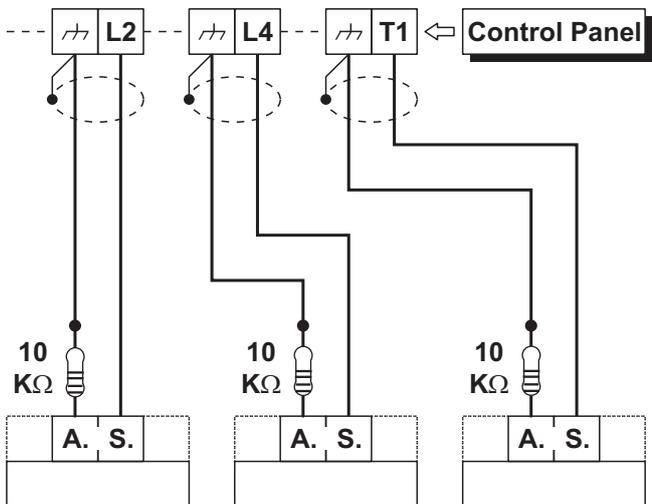
**Figure 18** Connecting 3 Tamper contacts to three 24h Zones with SEOL Supervision — the [A.S.] terminals represent the Normally Closed Tamper Contact of the device.
