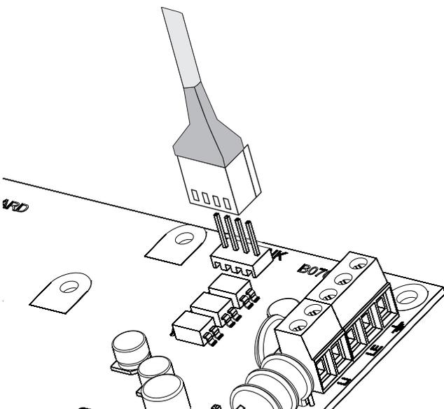
**Figure 24** PC-Link connection.
