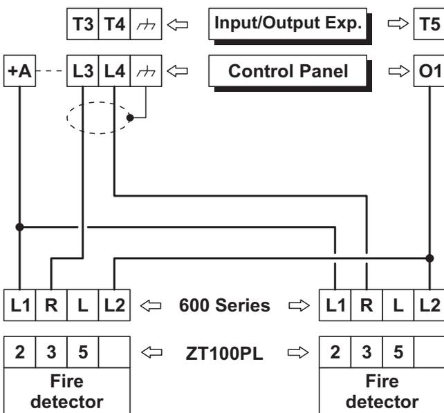
**Figure 13** Connecting 2 Fire Detectors to a Zone with Normally Open supervision (without diode).
