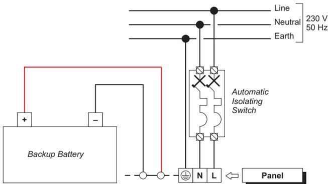
**Figure 21** Connecting the Mains power.
