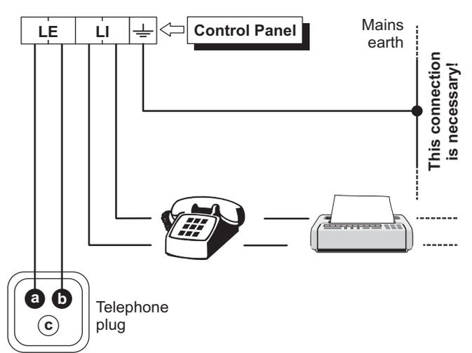
**Figure 19** Connecting the Telephone Line to the Control Panel.
