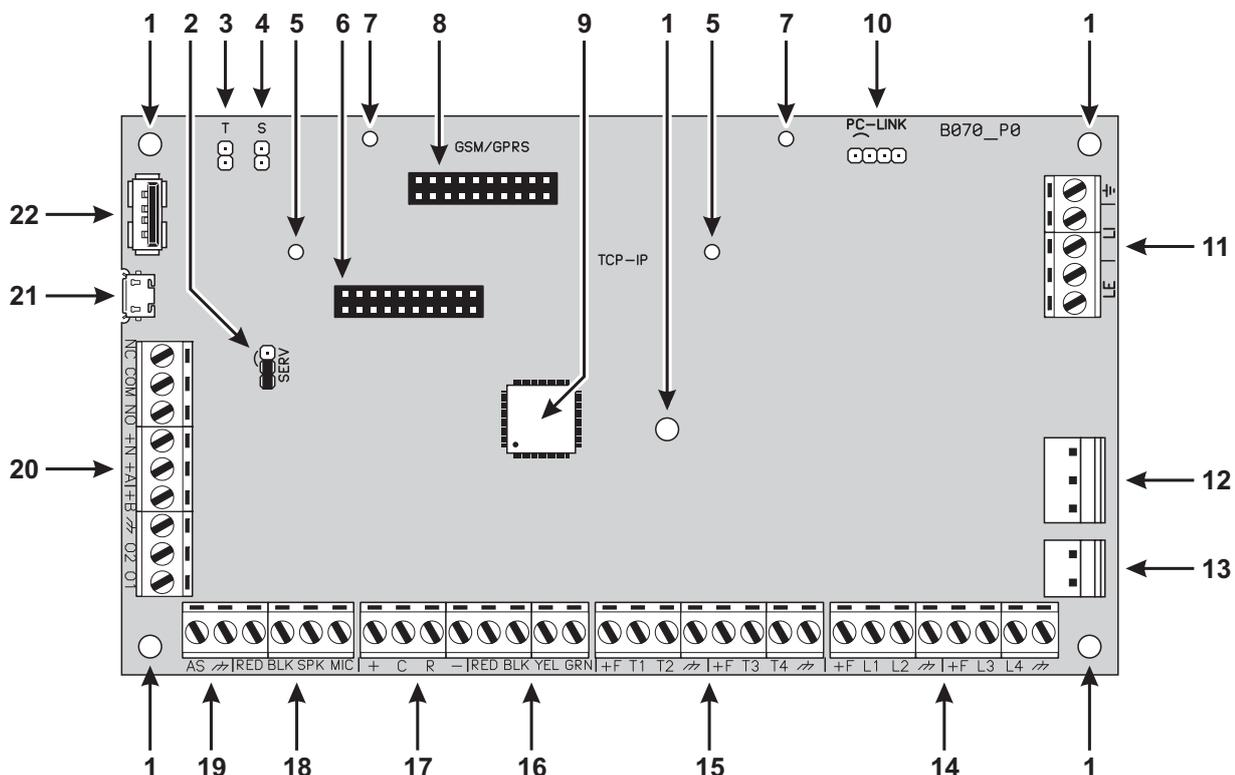
Figure 1 ABSOLUTA Main Board parts.
