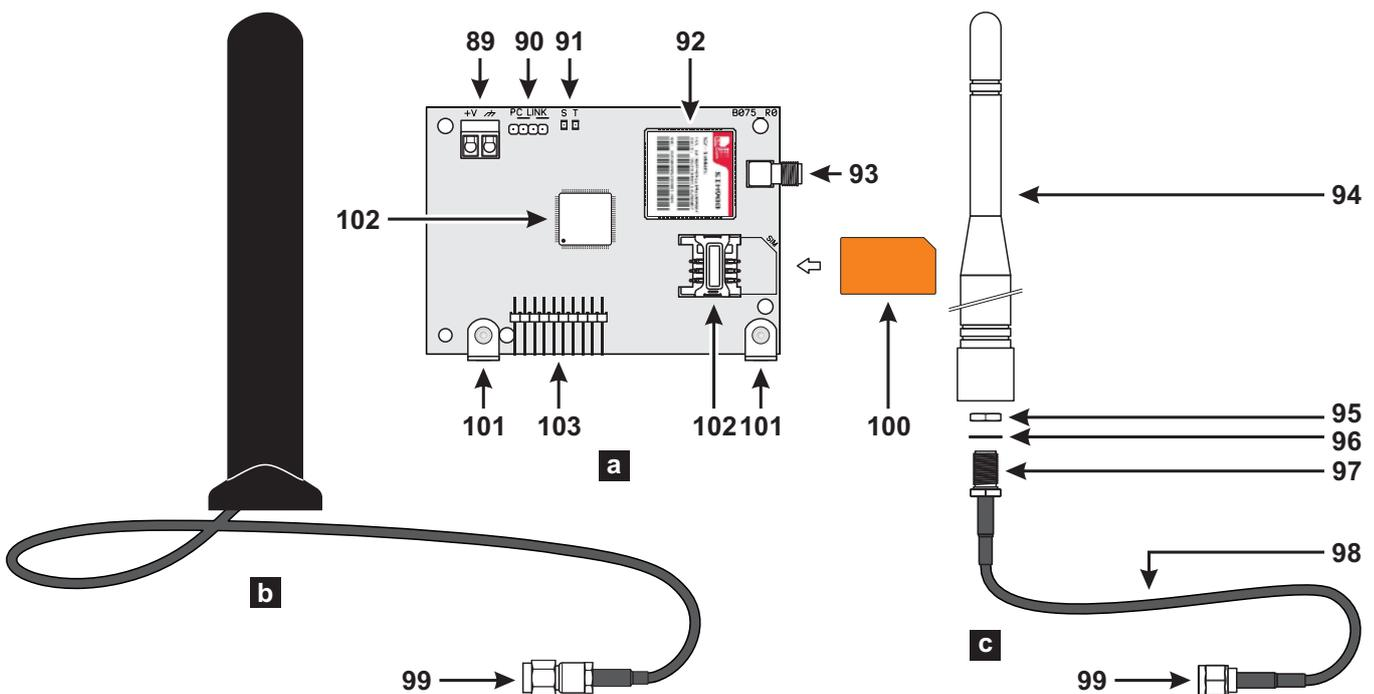
**Figure 6** Parts of the **ABS-GSM** Module (a), of the **BGSM-100CA** antenna for metal box (b), and of the **ABS-AK** antenna for plastic box (c).
