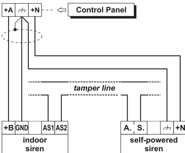
**Figure 15** Connecting a Self-powered Siren and an Indoor Siren to Control Panel Output no. 1.
