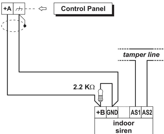
**Figure 16** Connecting an Indoor Siren to a Supervised Output on the Control Panel.
