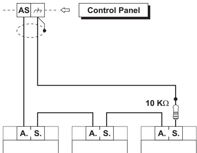
**Figure 17** Connecting 3 Tamper contacts to the Control Panel Tamper Line — the [A.S.] terminals represent the Normally Closed Tamper contacts of the device.
