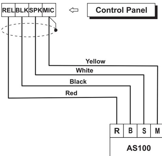
**Figure 20** Connecting the AS100 to the Control Panel.
