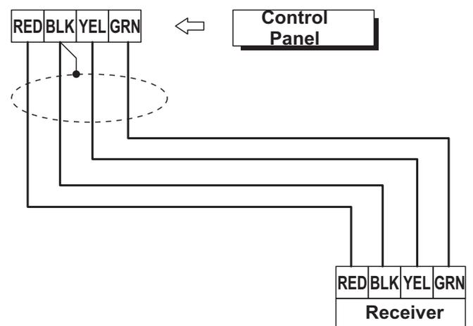
**Figure 26** Connecting the Receiver to the Control panel.
