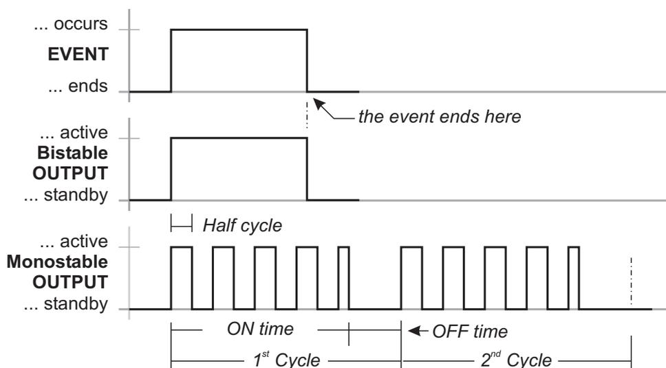
**Figure 23** The Effect of the **Oscillation** and **Cycle** options on Bistable and Monostable Outputs
