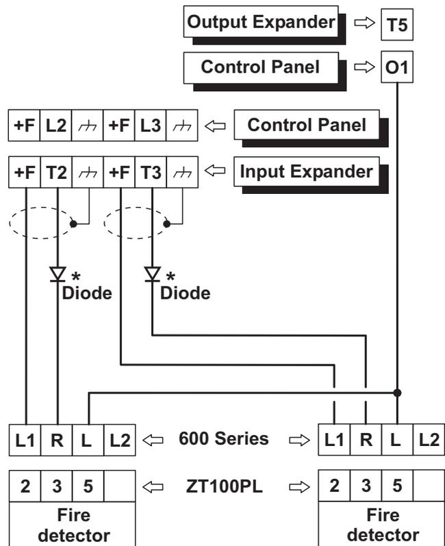
**Figure 14** Connecting 2 Fire Detectors to a Zone with Normally Open supervision (\* with series 600 ONLY).
