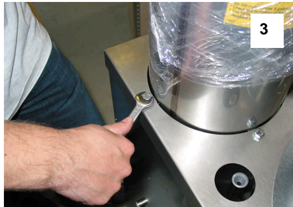
Center brackets and fit the three screws with washers
