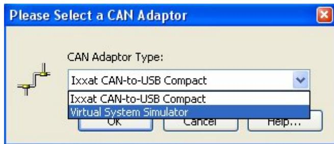
You will then be prompted to select a CSV file which contains all the information needed on the number and type of jacks, power pack arrangement, jack speeds, jack loads, etc.. The DL-P40 then uses this information in place of the information that it would normally receive from the CAN nodes. A number of example simulation files are automatically loaded to the desktop when you install the DL-P40.
