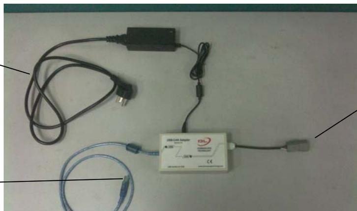
CAN communication line to the first power pack CAN node
