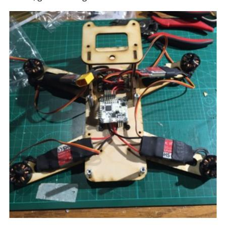
Once the motors have been bolted to the arms with the included 6mm M3 zinc steel machine screws, the ESC's have been zip-tied, and the rest of the
