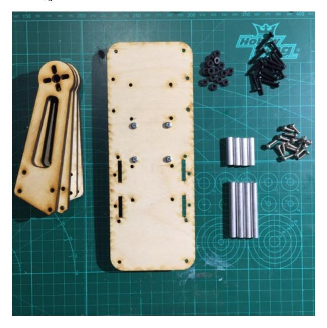
Install the standoffs by screwing in from the underside of the plate, as shown below. The definition of "underside" is up to you; the plate is symmetrical down the center, so either way up works just fine. Adding a dab of blue (removable type)
