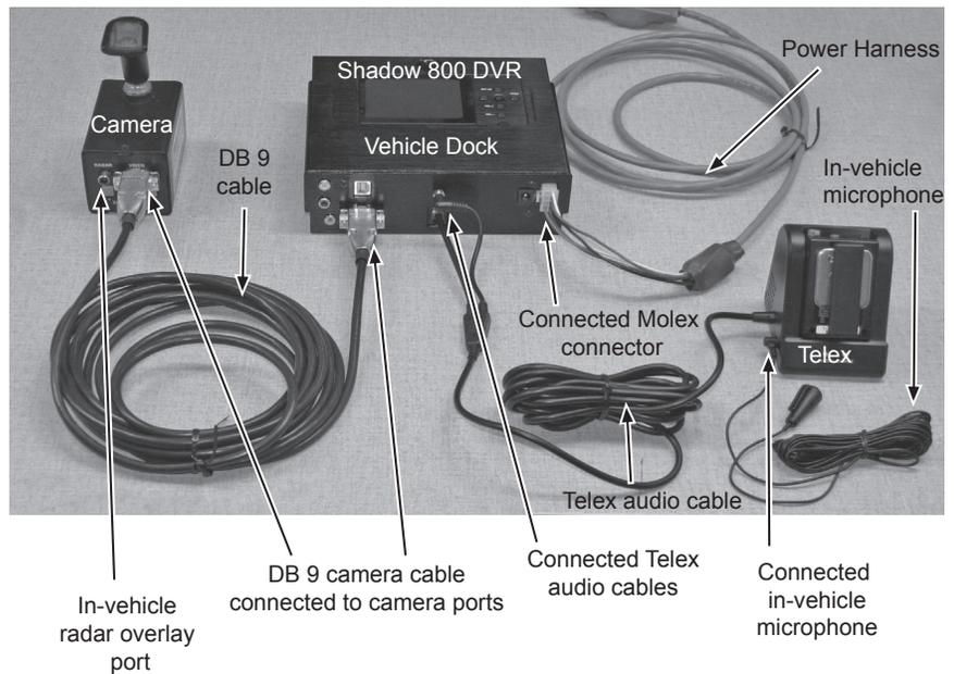
Figure 2 Connected cables
