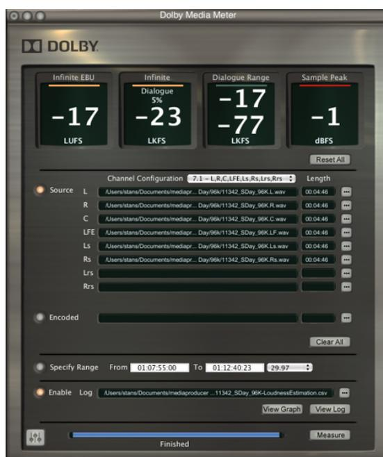
**Figure 1-1** Stand-Alone Meter Measuring a Set of Source Files
