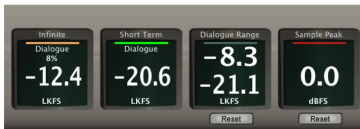
Figure 3-2 Measurement Pane Showing Tenths
