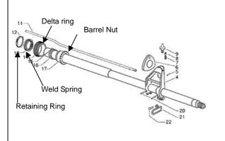
Step 01: Dissemble original M4 hand guards, outer barrel, Delta ring, Step 04: Insert PA07(gas tube) into the hole on PA04 (flash hider) and using spring pinto lock it, Then, put the whole set on to PA03(barrel) and
