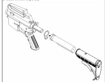
Step 05: Install PA05 onto rifle body and use screw to lock the adapter. Turn PA06 (tube) counter-clockwise onto the adapter.
